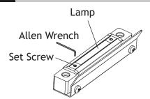
Using an Allen wrench, loosen the set screws on the ends of the lamp, then rotate the lamp to the desired direction. Always tighten the set screws after adjustments.
