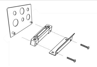
Pass the screws through the holes on the top of the fixture and into the mount. Hand tighten both sides, then firmly secure both screws with a screwdriver.
