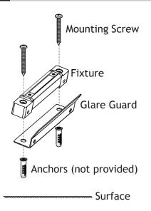
Pass the mounting screws through the holes on top of the fixture and mark both points on the desired mounting location. Drill holes using the marks, then insert the anchors (not provided) into the drilled holes.
